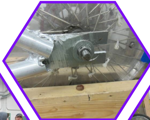
The rear wheel mount on correctly
