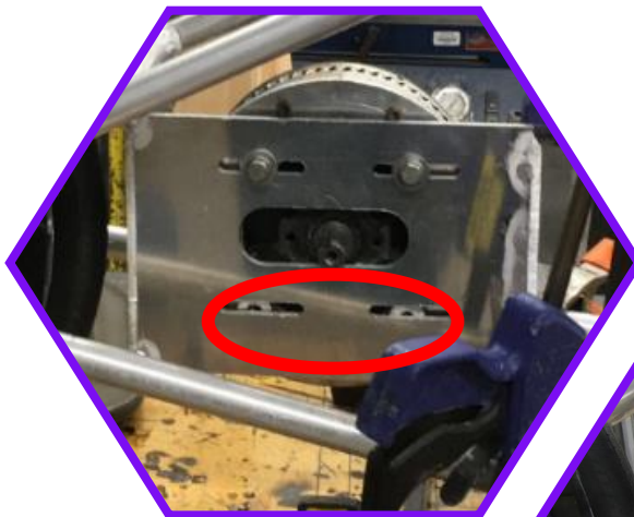
The new motor mount that didn't fit
