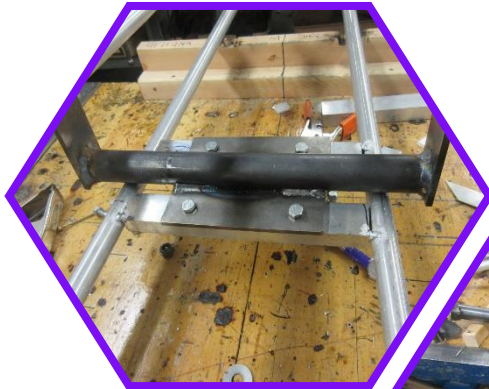
The middle axle section attached to the car
