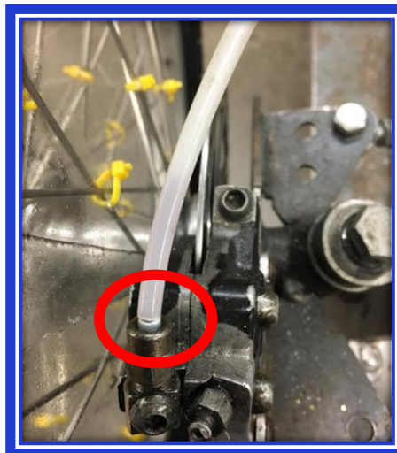
The cracked brake line
