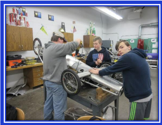
Assistant crew chief Mathew along with mechanical engineers Avery and Anthony, putting on the belly panels
